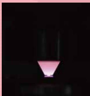
Plasma spot generation (diameter 1mm)
